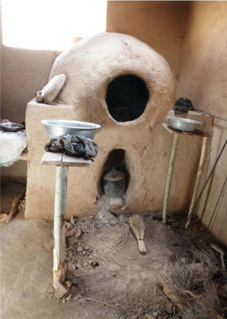
Traditional tandoor oven for baking bread: shrubs are used for fuel, fire is placed in the same chamber as the bread; smoke escapes into the room (Photo: Helvetas)
